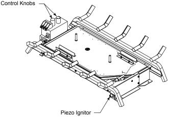
Figure 30 -Burner Controls
