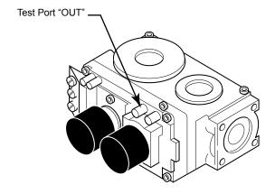
Figure 13 Pressure Test Point Location Millivolt Control
