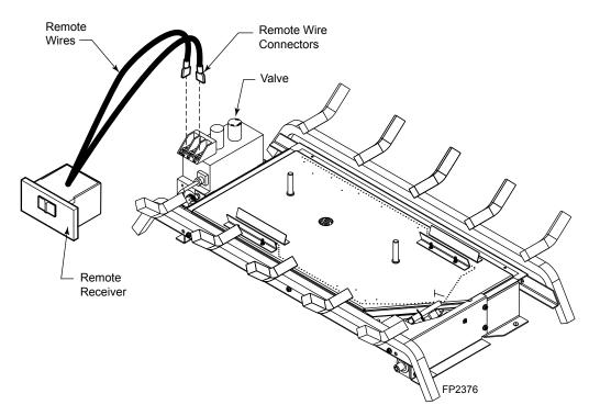
Figure 15 -Install Remote Receiver
