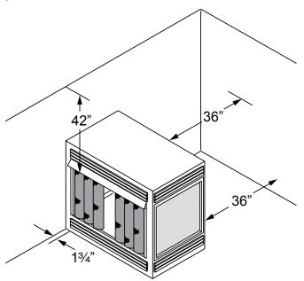
Figure 3 - Sidewall and Ceiling Clearances
