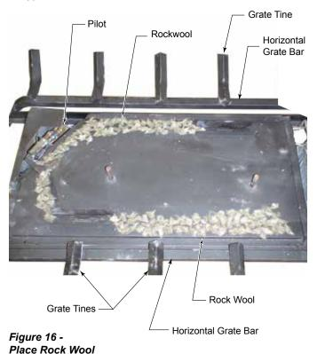
DO NOT sprinkle volcanic rock on the logs, around the pilot, or on or near burners. This may cause sooting. Place volcanic rock only on the floor of the fireplace.
