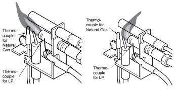
Figure 27 -Correct Pilot Flame Appearance
