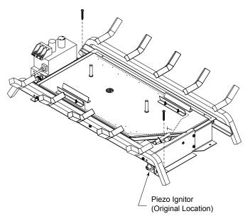
Figure 11 -Secure Burner
