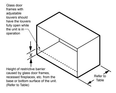
Figure 2 - Reference Drawing of NBST27 Log Set in an Enclosure
