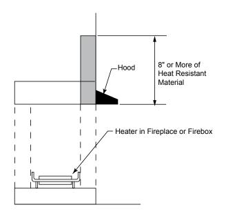
Figure 5 -Measure Heat Resistant Material for Mantel
