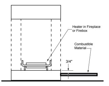
Figure 8 - Minimum Clearance above Combustible Flooring
