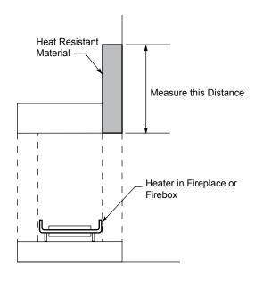
Figure 4 - Measure Heat Resistant Material
