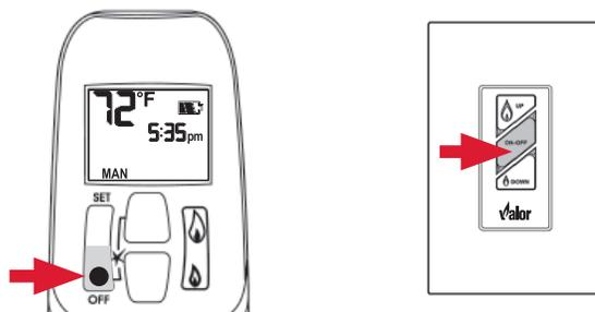
If the flames are on, they go down and you hear the valve motor wind down. You hear a clunk and a beep indicating that the valve has received the signal from the remote control.
