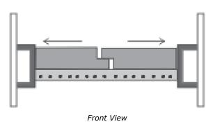
4 . Install the 2 front secondary air tubes with pliers and hammer to lock them into place, as shown below.
