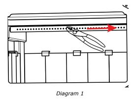
5. To reinstall or replace, first slide left side of tube into hole on left side air channel. Align tab on right side air channel with notch on right hand end of air tube. Firmly grip center of air tube with vise grips, use hammer to tap vise grips from left to right until the tube bottoms out into the air channel on right.
